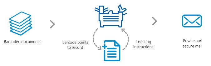
The reference file is used to control and constantly verify pages are accurately folded and inserted.
