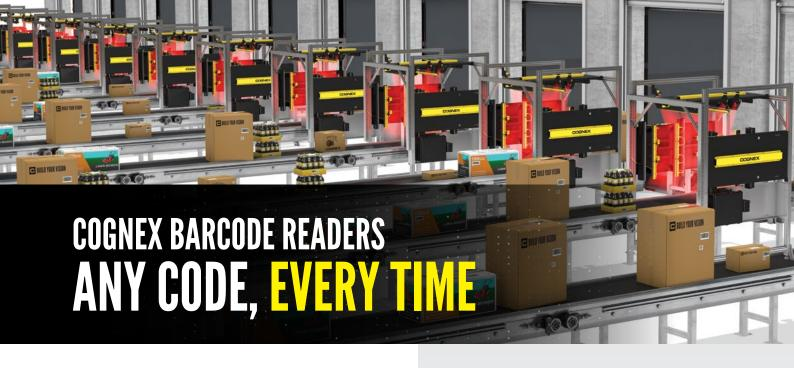
Nearly every product uses a 1D or 2D barcode to automate and simplify identification and data capture. The basic process in reading codes is to 1) illuminate the code, 2) locate the code, and 3) extract the data. Organizations must be able to read codes quickly and accurately for maximum efficiency and throughput.
