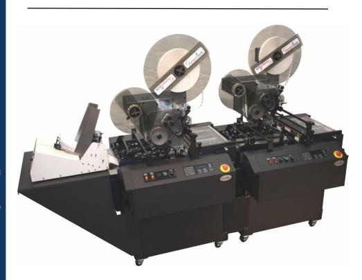
The Ameritek Tabber can also be configured as a Dual Headed Tabber. This system can tab on the leading (toe) and trailing (heel) edges of a booklet in a single pass. The Dual Headed Tabber can run in-line or off-line as a system, or the Tabbers can be unlocked and used as stand-alone units.
