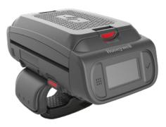
The ergonomic 8690i Wearable RFID Mini Mobile Computer delivers essential workflow information directly to the worker's line of sight and enables input to support common workflows with a single device. Eliminating wasted motion with always-at-hand, ergonomic RFID reading and scanning drives efficiency in high frequency workflows.
